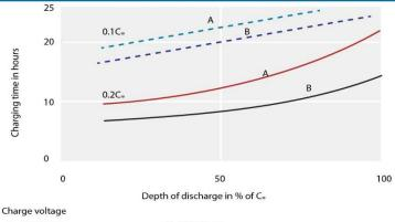
A - 2.25 V/cell State of charge 100% B - 2.40 V/cell State of charge 90%
