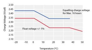
For continuous charging we recommend a voltage of 2.25 V The charging voltage must be compensated to the curve for a continuously different battery ambient temperature
