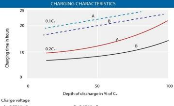
A - 2.25 V/cell State of charge 100% B - 2.40 V/cell State of charge 90%
