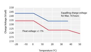
For continuous charging we recommend a voltage of 2.25 V The charging voltage must be compensated to the curve for a continuously different battery ambient temperature
